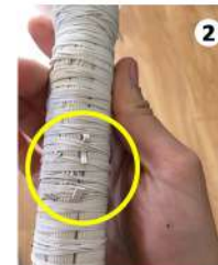
Exemple of damaged core strings
